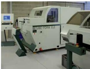
Tube processing specialist HMD Ltd's new 21,000 sq. ft. building in Hoyland Road, Sheffield, has nearly three times the floor area of its current unit and is home to a four-machine tube processing cell supplied by BLM GROUP UK Ltd. This new cell is dedicated to producing copper components and comprises three new machines – BLM Process, BLM Dynamo-E tube bender and BLM Tube-Form ELE tube end former – along with an existing
